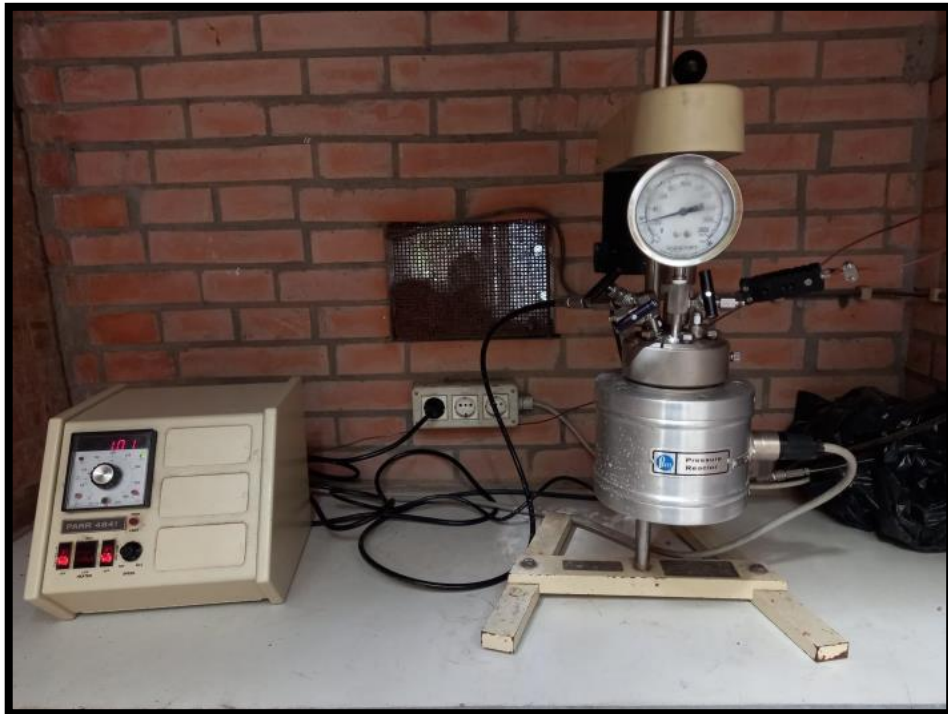
Synthesis of Ruthenium carbonyl precursor in an autoclave (high-pressure reactor).
