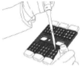
1. Add 100  $\mu$ l assay diluent to each carrier well followed by 100  $\mu$ l of prepared sample/control/standard.
