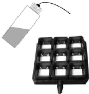
5. Decant liquid and wash each well. Perform 2 quick washes and 4 two-minute soaks. Decant liquid and tap on lint free paper.
